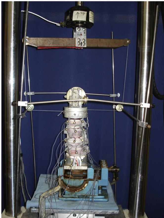
Fig. 3. Apparatus used with a system of cables and pulleys imparting non-destructive, non-constraining torques in conjunction with a standard servohydraulic test system.
