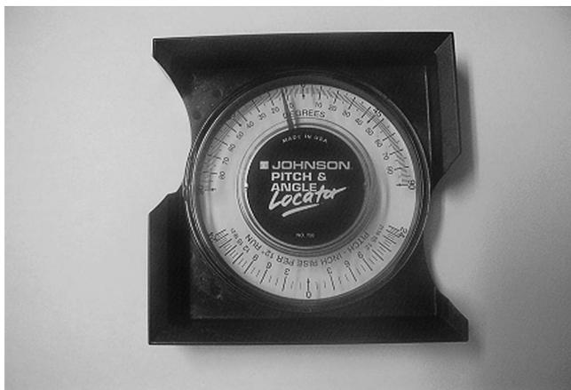
**FIGURE 1.** Angle measuring device by Johnson Level & Tool Contractor Pitch and Slope Locator 750 (Johnson Tools Mfg. Co.Ltd., Jiangsu, China).
